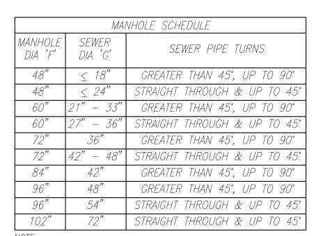
MANHOLE MANUFACTURER TO PROPERLY SIZE AND DESIGN STRUCTURES TO MAINTAIN MANHOLE STRUCTURAL INTEGRITY.
